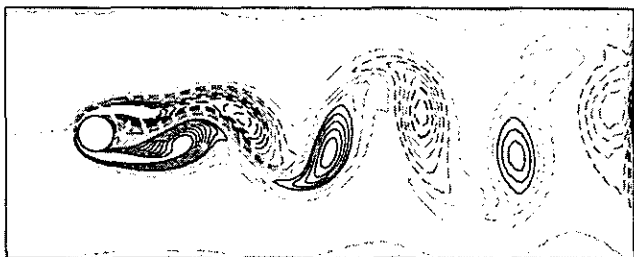
FIG. 4. Flow past a cylinder, vorticity, max = 26, min = -26.
